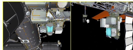
Figure 6: Sample external stowage location specifications. The left picture is a flex hose rotary coupler on ESP 2, position 7. Its orientation is aft, port, nadir, so the full spec is ESP0207aftPrtNad. The right picture is that of a pump module assembly on ELC01. Its location spec is ELC0107fwdStbNad.
