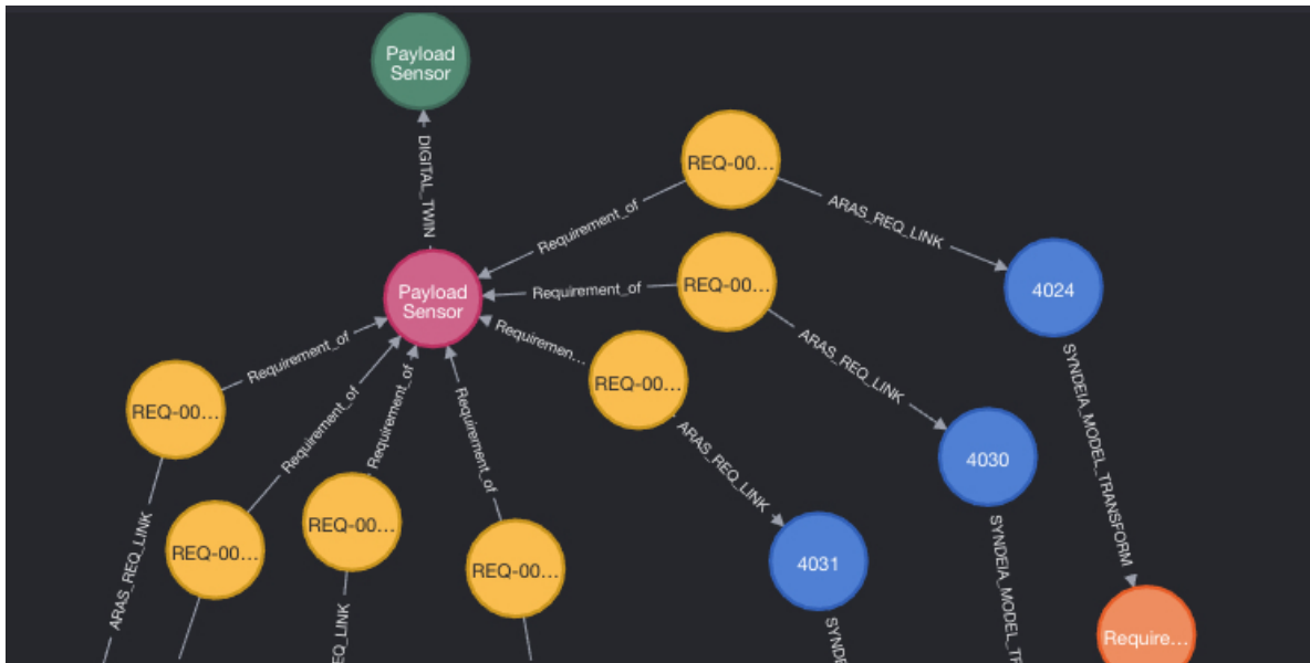
Figure 14: Part of the traceability graph generated to show links to the Payload Sensor explored in demonstration 3. The green Payload Sensor node is an Aras digital twin, the pink Payload Sensor node is an Aras part, the yellow nodes are Aras requirements, and the blue nodes are DOORS requirements.
